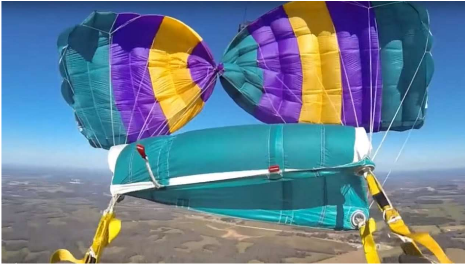
Photo 1 – A suspension line (shroud line) has gone over the top of the canopy
