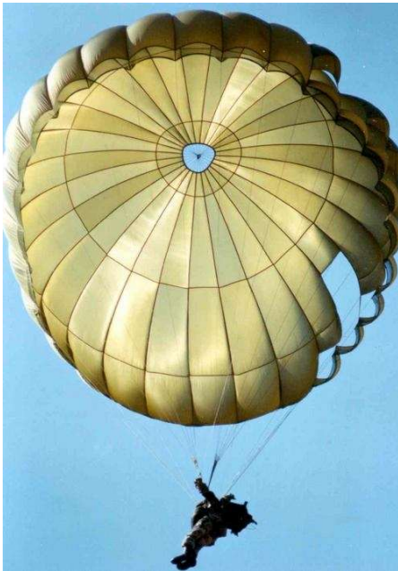
Photo 4 – The canopy has open sections allowing air to spill out and propel the parachute forward allowing some control over the landing area.
