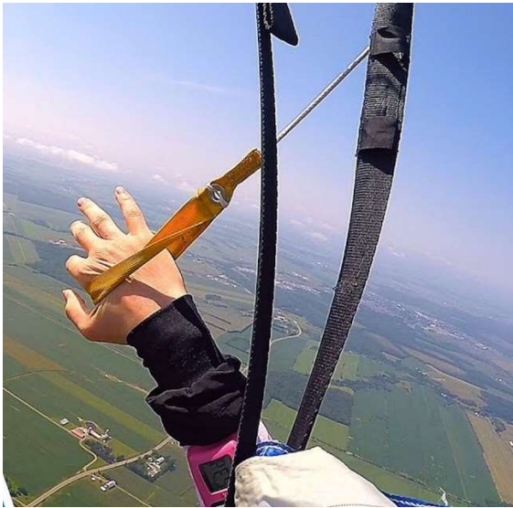
Photo 3 – The toggles for steering the parachute may look like canvas loops, some canopies do not have toggles and you pull on the riser to steer.
