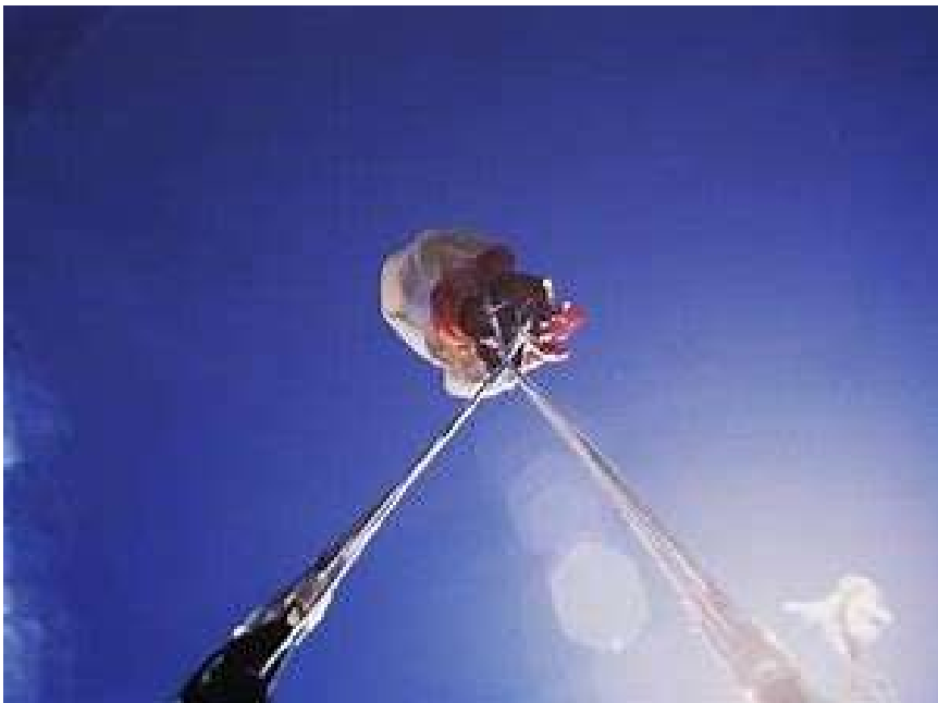
Photo 2 – The risers have become twisted.
